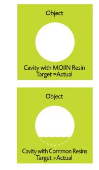
Tailoring of the 3D printing resin in terms of  $E_c$  and  $D_D$  is key to achieve accurate objects. In a high  $D_D$  and lower  $E_C$  situation, as shown on the left image, the area of overcured material is larger. This leads to inaccurate object dimensions. In the case of small scale hollow structures these might be blocked by overcured material.
